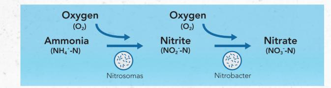
Through biological oxidation, (Nitrification) in the bioreactors, by pumping in high levels of Oxygen, Nitrosomonas bacteria convert Ammonium to Nitrite. These Nitrifiers are found in our bioreactors.
